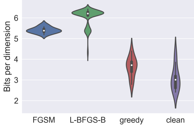
Figure 3. The bits-per-dimension distributions of purified images from FGSM adversarial examples. We tested two purification methods, L-BFGS-B and greedy decoding, the latter of which is used in PixelDefend. A good purification method should give images that have lower bits per dimension compared to FGSM images and ideally similar bits per dimension compared to clean ones.
